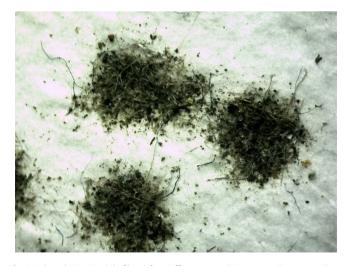
Fig. 2. Microplastics (mainly fibers) from effluent water (Wastewater Treatment Plant-Two Harbors, MN).
