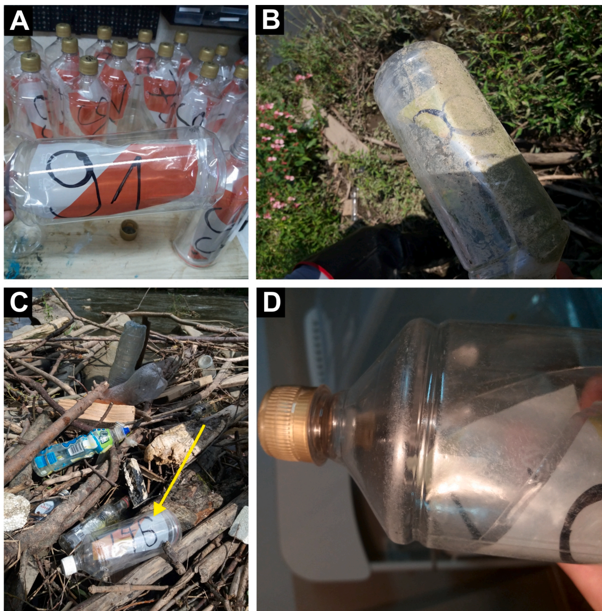
Fig. 3. Tagged 1-litre PET bottles used in the experiment. Tagged bottles before (A), during (B, C) and after experiment (D). Last photo (D) indicates small cracks formed on the bottle surface during 52 days of transport in the river channel.
